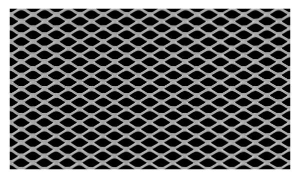
LW Aperture:9.50mmStrand Width:1.30mmSW Aperture:5.00mmThickness:0.90mmWeight:2.42 kg / m2Open Area:66%
